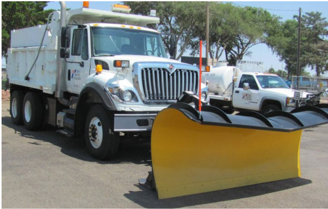
Figure 3-4. The Snow Plow is an attachment for a six- and 10-cubic yard truck. It is used to remove snow from the pavement.
