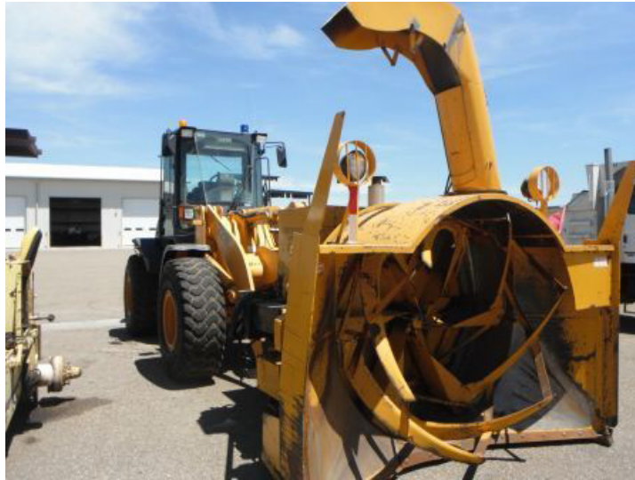
Figure 3-8. Snow blower is an attachment that is used to remove large quantities of snow.
