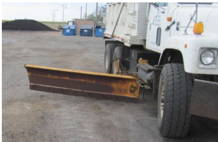
Figure 3-7. The snow wing attachment provides extra width on a motor grader or truck for plowing two lanes at a time or picking up a lane and a shoulder at the same time.
