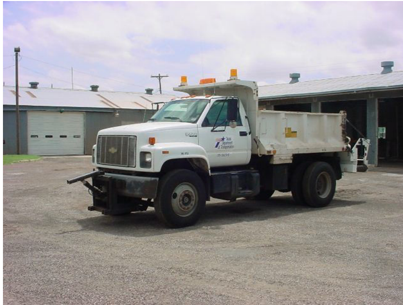
Figure 3-1. Dump trucks are the workhorses of TxDOT snow removal. Snow plows are mounted to dump trucks and are used to push the accumulated snow off the roadway. Spreaders are also mounted on dump trucks to facilitate the spreading of materials for snow and ice control.
