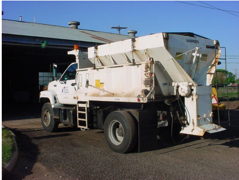
Figure 3-5. The V-Box Spreader is an attachment for a dump bed truck. It is used to accurately put out applications of de-icing materials on bridges and icy spots. These spreaders can either be hydraulic or gasoline operated.
