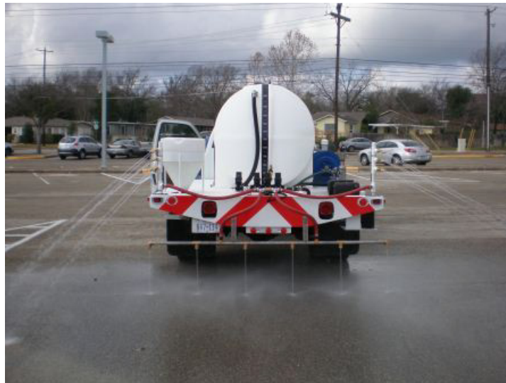
Figure 3-9. The herbicide rig is used to apply anti-icing liquids prior to an approaching storm. It is also used for de-icing applications during the storm.
