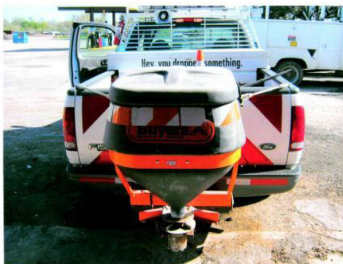
Figure 3-10. Pickup applicators are used to apply anti-icing liquids (top) and granular (bottom) materials prior to an approaching storm to small areas such as bridge decks, on and off ramps. They are also used for de-icing applications during the storm.
