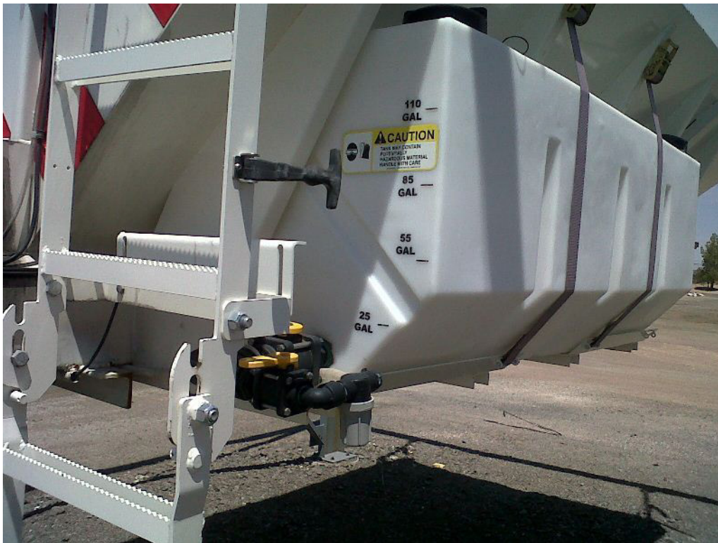
Figure 2-2. A saddle tank is a useful means of pre-wetting solid chemicals.
