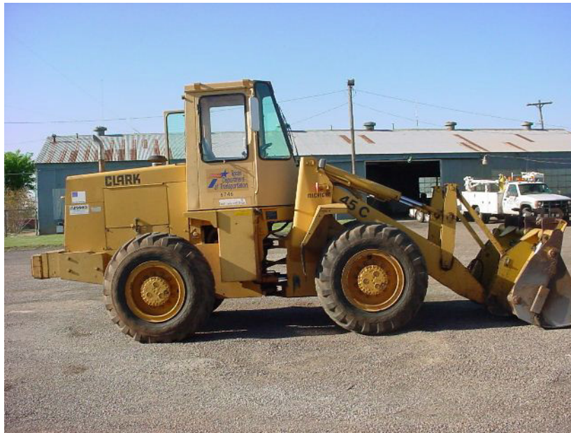
Figure 3-3. Loaders are a vital piece of equipment during a snow and/or ice event. They are used for loading material on the trucks to fight the ice and snow. They are also used to clear intersections and driveways.
