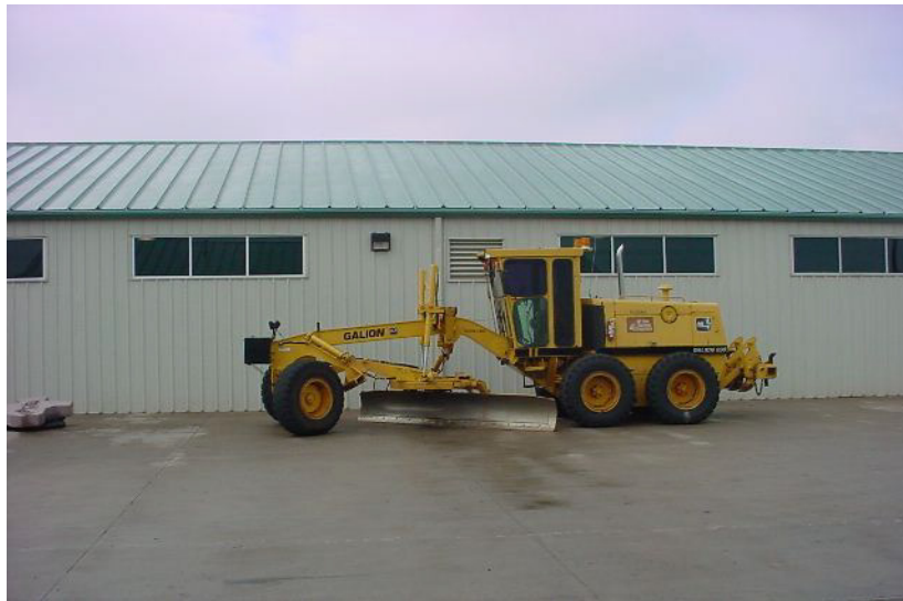
Figure 3-2. Motor-grader (maintainer) - This may be the best piece of equipment we have for snow removal. It does not require any other attachments to do the job. This piece of equipment is self-contained and ready to go.
